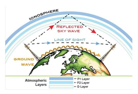
The D layer is the lowest electrified layer of the ionosphere. This is the layer that causes problems for broadcasting. During the day, when there are a lot of solar flares, radio waves get absorbed by the D layer, which is why signals do not transmit very well during the day. Solar flares are intense variations in brightness that occur when built up magnetic energy is suddenly released. The D layer almost completely disappears at night, allowing the F layers to reflect radio signals.
